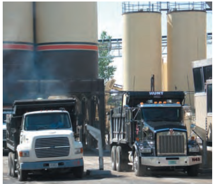
The difference between hot mix and warm mix is very evident at the point where the paving material is loaded into trucks at the plant. Hot mix produced at 320° F is in the truck on the left. Warm mix at 270° F is on the right.
