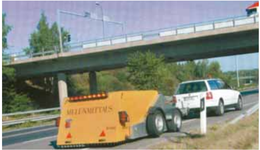
Figure 2 – Finnish CPX Noise Trailer The NCAT trailer is being used to measure road noise close to its source.
