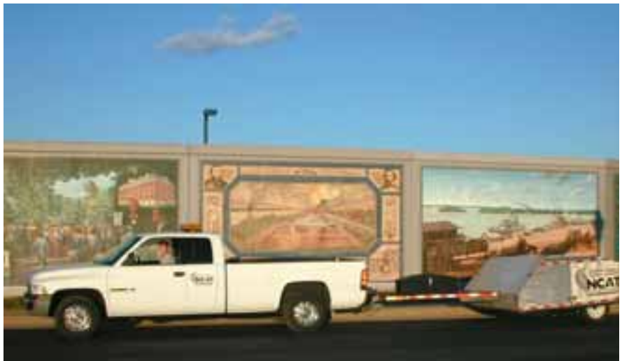
Figure 3 – NCAT close proximity trailer Measuring road noise at a standard distance.
