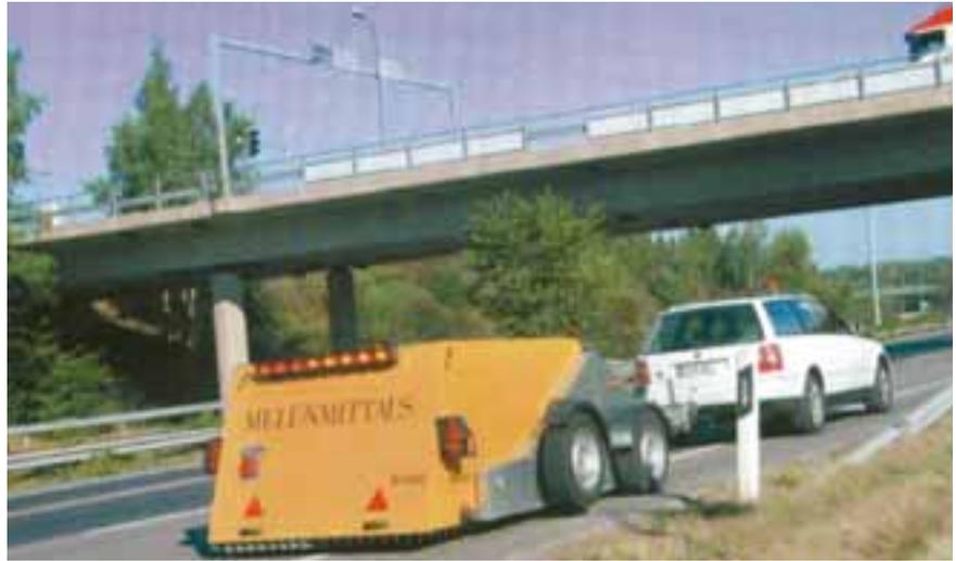
**Figure 2 – Finnish CPX Noise Trailer**
