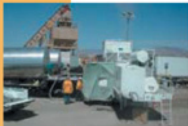
The equipment for adding crumb rubber to Hot Mix Asphalt can be set up at a typical HMA plant.
